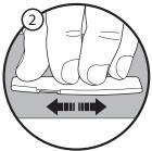
Check if the Graph Tech saddle fits into the slot, without forcing it. If it's too thick, place a 240 to 600 grit sand paper on a flat surface and sand the sides of the saddle until it fits in the slot snugly but is easily removable. You may have to reduce the length also.
