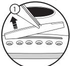
Remove the strings and bridge pins. The saddle should lift out easily. If you find it is glued in, get a competent guitar tech to complete the replacement. Do NOT pry it out as you may take some wood from your bridge with it. Once removed, clean the slot of any debris.
