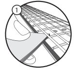
Determine correct string height, by measuring the gap between the top of the twelfth fret and the bottom of the low E string. It should be around 0.125" (3mm), or about a stack of 12 business cards if you don't have a ruler. For the high E string, the gap should be around 0.080"(2mm), or about a stack of 8 business cards.
