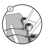
**Remove your old bridge pins** using your fingers or a pin puller like the one on the end of most string winders.
