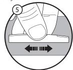
Sand the bottom of the saddle up to the line, keeping the bottom flat and square to the sides. Work in small increments and check your work frequently so you don't remove too much material
