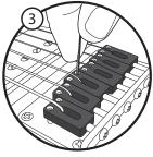
Adjust string height using the supplied allen key to lower or raise your saddles until correct string height is acheived. Be sure to adjust both height adjustment screws equally to keep the saddle level. Tune guitar to concert pitch after each adjustment. Repeat for each string.
